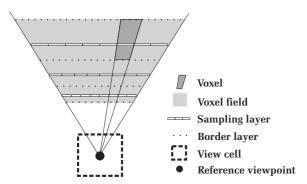
Figure 2: Layout of the voxel field for a view cell.
