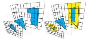
**Figure 6:** Left: the polygon edge clipped on the border plane is not represented completely in both adjacent sampling layers. Right: by drawing the outline of the clipped polygon explicitly (light pixels), a complete representation of the clipped edge is generated in both sampling layers.
