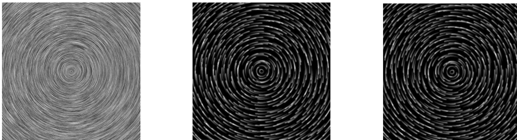
Figure 1: LIC image of circular flow (a), OLIC image with clockwise flow (b), OLIC image with counterclockwise flow (c) [WeGr97b]
