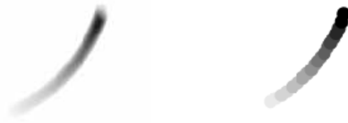
Figure 2: Exact trace of a droplet with OLIC (a) and approximated trace of a droplet with FROLIC (b) [WeGr97b]
