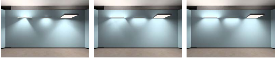
Fig. 1. Photometric point lights (left), a typical simplification of photometric area lights used in real-time rendering systems. Our real-time technique (middle) provides a well-defined illumination in the near-field of the light sources, closely resembling the reference solution (right) rendered with 5000 point lights.
