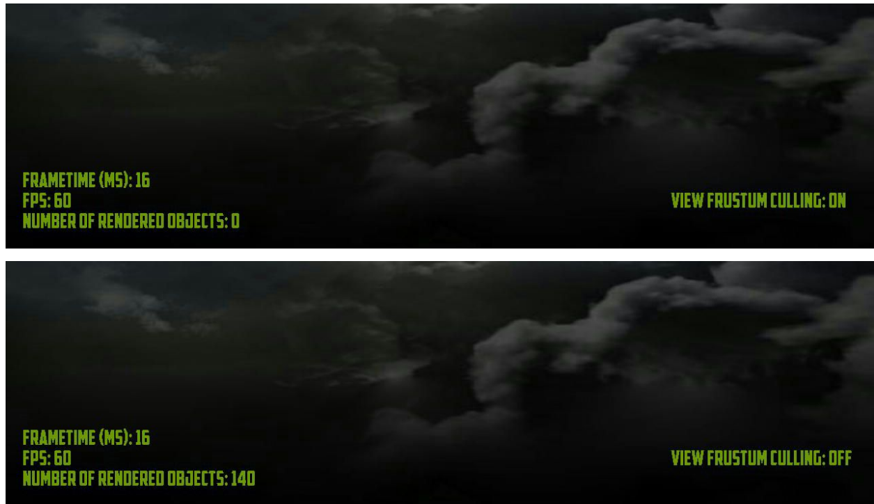
Fig.7.: View frustum culling on ( top ) and off ( bottom )
